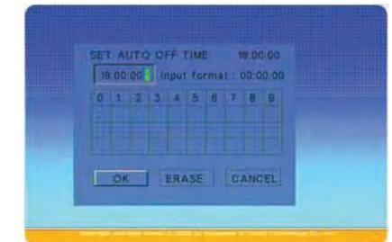
The MP50A will now turn on and off automatically on a daily base at your preset time. To turn it OFF, go to the Advanced Setup menu, select Auto ON/OFF and deactivate this option.
