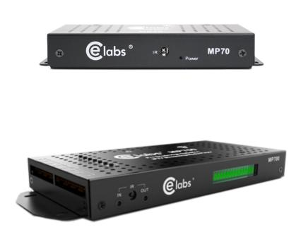
These players are small ASIC based processors running a Micro Kernel. These players **ARE NOT** PC or Android based and are designed for their one unique task only.
